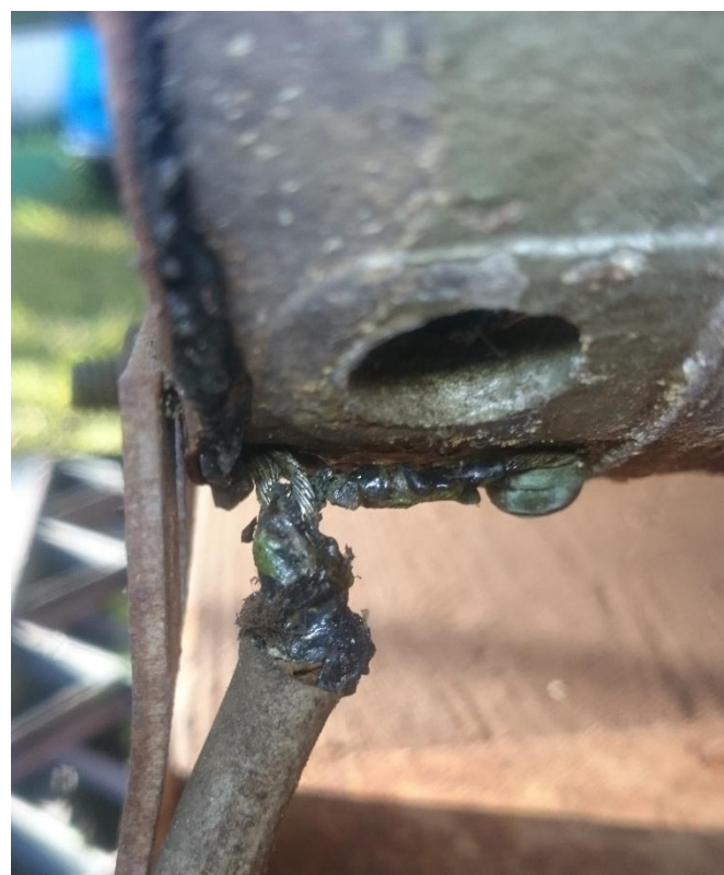
Close up of the resulting short circuit at the motor
