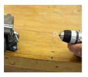
prong wires and stand them up in the holes. The wires support themselves, soldering is easy, and the joint is stronger because of the increased soldering area.
