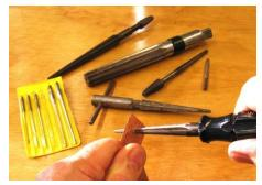
wire just fits. For larger hole sizes in sheet metal up to 14 ga, I really like the reamer with the black handle. It makes quick work of sizing holes from about 3mm to 12mm. You can find them in well-equipped hardware stores. You may never use the large diameter reamers, but when sawing out some rings from 4mm thick sheet, I found they worked well for rounding and sizing the hole.
